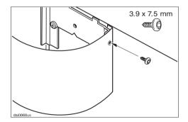
Push the chimney extension flush against the ceiling and use 2 of the small screws to attach it to the top of the retaining plate.
